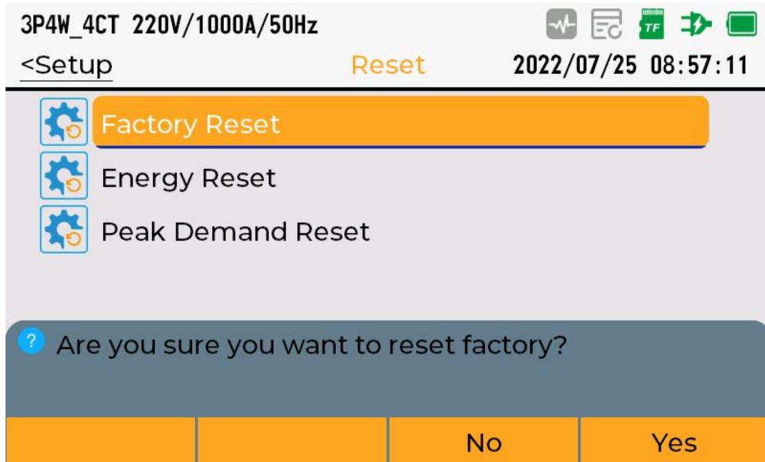
Figure 5-30 Operation confirmation interface
