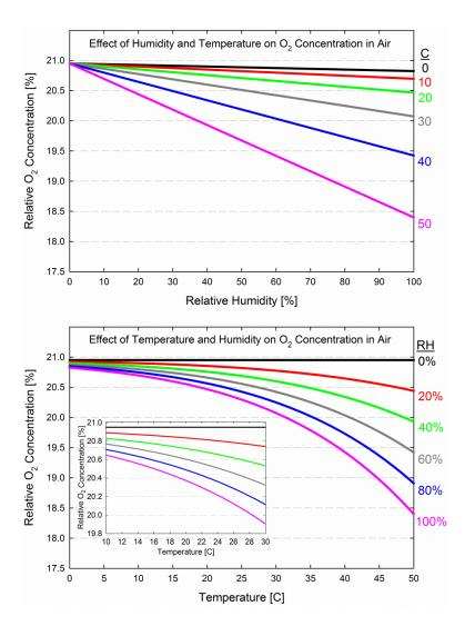
A) Relative humidity effects on relative oxygen concentration shown as a function of relative humidity at temperatures increments of 10 C and B) as a function of temperature at relative humidity increments of 20 %. The air in soil is typically always saturated with water vapor (100 % relative humidity) unless the soil is very dry.
