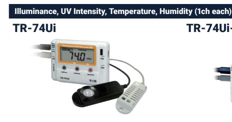
Illuminance: 0 to 130 klx UV Intensity: 0 to 30 mW/cm<sup>2</sup> Temperature: 0 to 55 °C Humidity: 10 to 95 %RH
