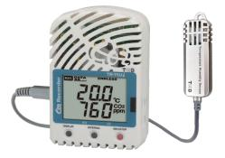
CO2: 0 to 9999 ppm Temperature: -25 to 70 °C Humidity: 0 to 99 %RH (above -20 °C)
