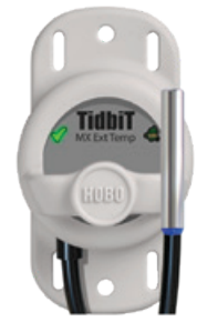
MX2205 External Temperature Depth rating 100 ft
