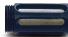
F5200B - sensor cover with filter from stainless steel mesh, suitable for moderately dusty environment. Filtering ability 0.025 mm.
