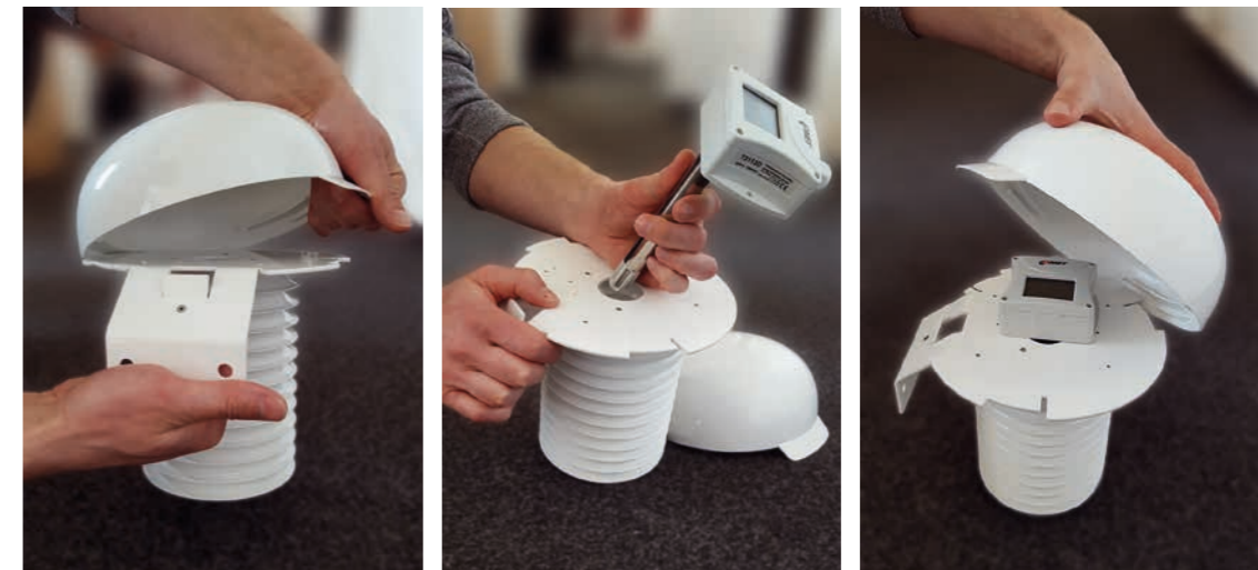
Mounting of sensor inside of COMETEO.
