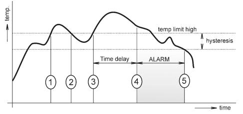
In Point 1 the temperature exceeded the limit. From this time, the time-delay is counting. Because at point 2 the temperature dropped below the limit value before the time delay expired, alarm was not set.
