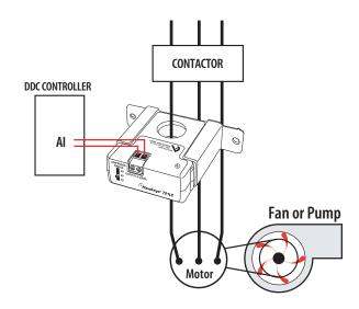
Note: This example diagram refers to the H721xC. Please see the H721xC and H921 installation guides for specific wiring information.
