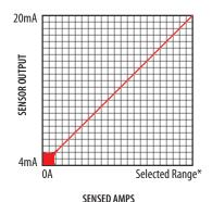
\*Factory calibrated ranges selected with the amperage range switch
